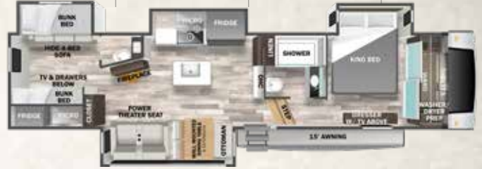
3325BH HITCH WEIGHT-2,130 lb. / GVWR-16,130 lb. / UVW-12,324 lb. CCC-3,806 lb. / LENGTH-38' 8" / HEIGHT-13' 6" / WIDTH-96"
